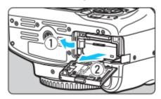
Move the tab on the left further to the left, and the battery should pop out a bit. Remove it all the way for safe storage or charging.
